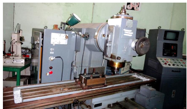
Fig. 1: Experimental Setup describing clamping of FSW plate
