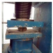
Fig. 5 Split tensile strength test
