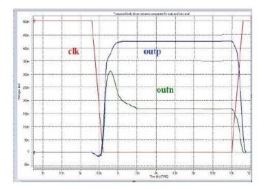
**Chart -2** Simulation of proposed body driven Dynamic Comparator
