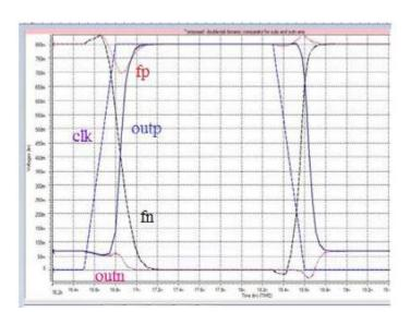
**Chart -1**Simulation of Modified Double Tail Dynamic Comparator
