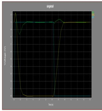
Fig. 2. Fleeting simulations of the conventional dynamic comparator for input voltage difference
