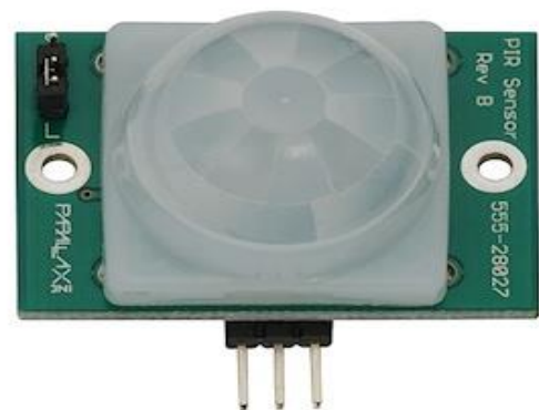
Fig -6: PIR sensor
