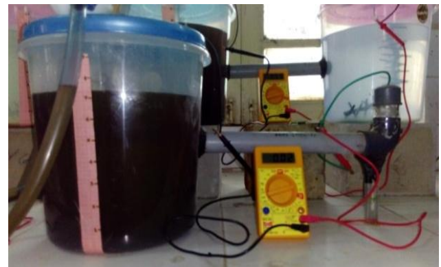
Fig-6: Experimental set-up of Single Chamber Air Cathode MFC
