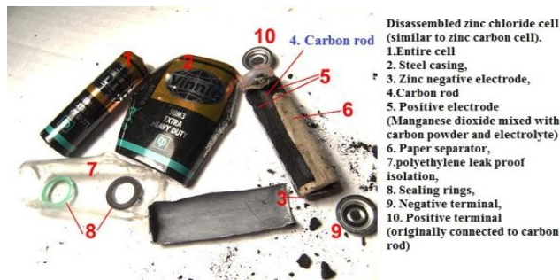
Fig-3: Extracted carbon rod from battery cell for preparing carbon brush
