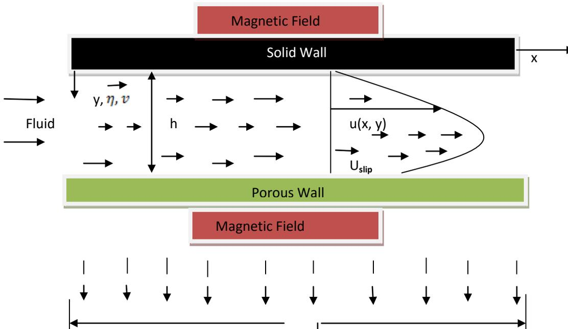
Fig. 1. The coordinate system used in the solution of the two dimensional steady State Navier-Stokes equation in Presence of Magnetic field
