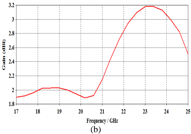
Fig -2: (a) Variation of reflection coefficient (S11) as a function of frequency (b) Variation of gain with frequency.
