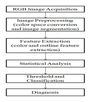
**Fig-2:** Processing flow of feature extraction and processing
