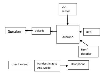
FigII.1: Block diagram of IVRS Based System
