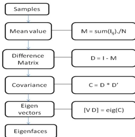
Fig - 1: PCA algorithm flow
