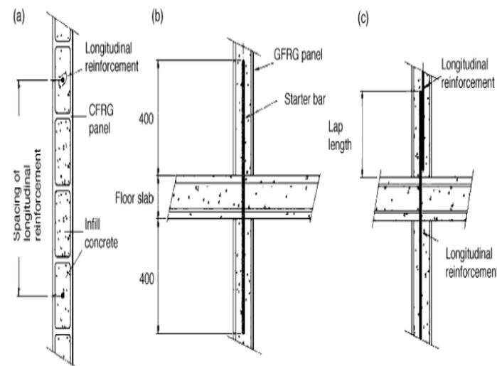
Fig.2: Connections between wall and floor. (a) plan, (b) vertical section of a starter bar connection, (c) vertical section of a continuous reinforcement.
