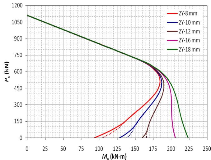
**Fig.5:** Pud and Mud interaction diagram for 1.25 m wide GFRG panel
