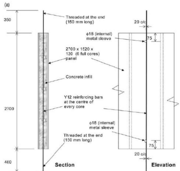
**Fig.6 (a):** Specimen with full length bars
