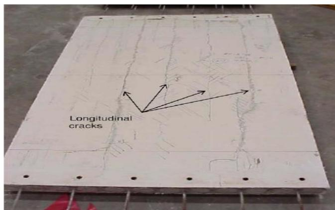
**Fig.4:** Typical Longitudinal shear failure
