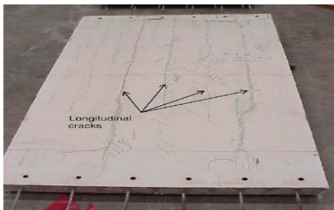
**Fig.4:** Typical Longitudinal shear failure
