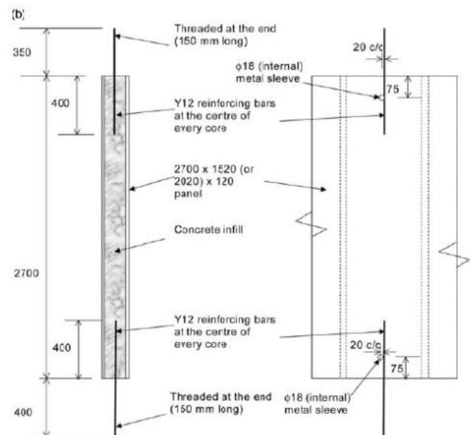
**Fig.6 (b):** Specimen with starter bars
