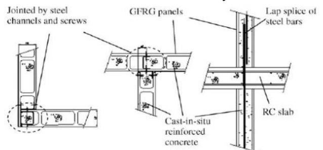
Fig.3: (a) Horizontal Joints (b) Vertical Joints
