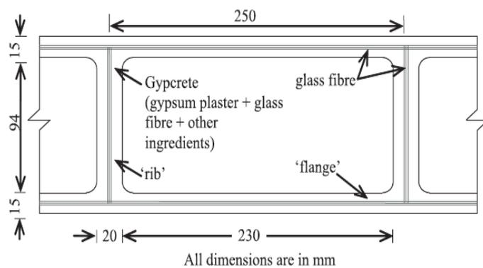
(b) Enlarged view of a typical cell of GFRG panel
