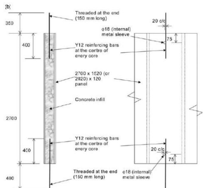
**Fig.6 (b):** Specimen with starter bars
