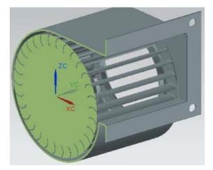
Fig -3: Sectional view of the fan
