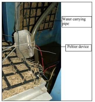
Fig -4: Peltier device
