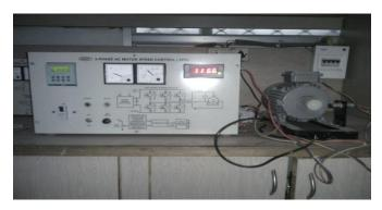
Fig -11: Hardware Model of Variable Frequency Drive
