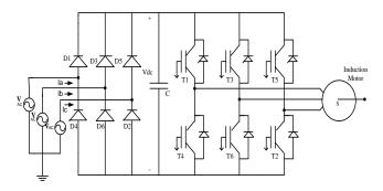
Fig -2: Equivalent circuit of Variable Frequency Drive
