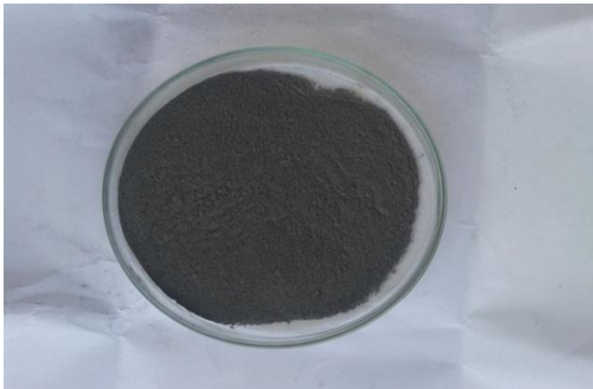
Figure-3: Bottom fraction from froth flotation
