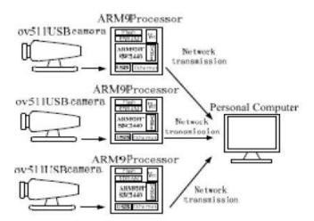
Fig -2: Structure of video capturing system
