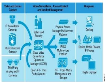
Fig -1: Architecture of video surveillance system
