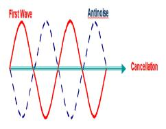
Figure 1. The mechanism of active noise cancellation control.
