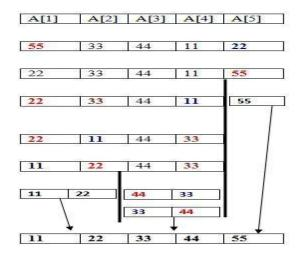
**Shell sort:** This sort was invented by Donald Shell in 1959. It is improvement over bubble sort and insertion sort. One way to implement is to arrange the data sequence in a two-dimensional array and then sort the columns of the array using insertion sort.
