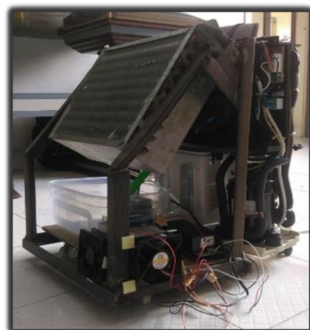
Fig -5: Final fabricated air cooling unit.
