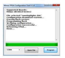
[3]Above snapshot shows that the program is fed to the spartan6 module kit.
