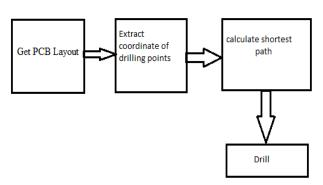
The first step is getting the PCB layout. This is simply done by the PCB design software. A simple enough task for beginner in a PCB designing as is our goal. Figure sample schematic of image file Once the image is obtained it is loaded into the MATLAB program which will extract the coordinates for plotting.
