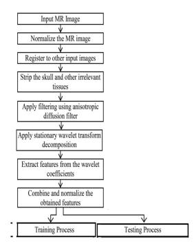
Fig- 1 : Flow diagram of the segmentation algorithm.
