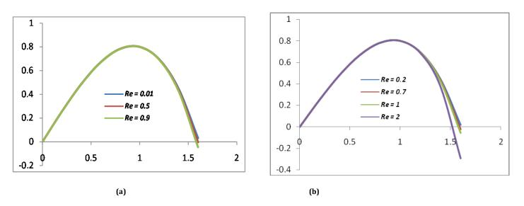
Fig. 2. Graph between dimensionless variable  $\lambda$  and fluid velocity  $f(\lambda)$  in the different Suction Reynolds Number.
