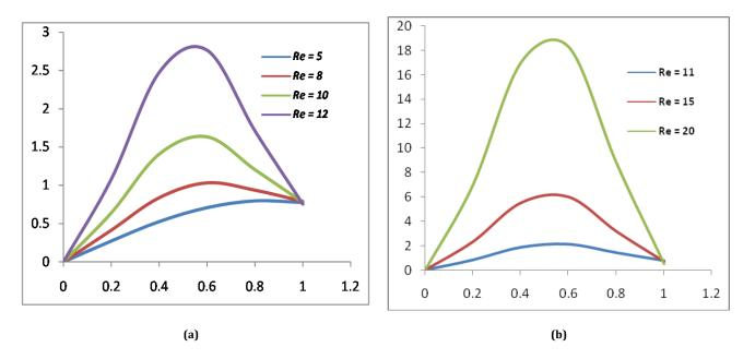
Fig. 3. Graph between dimensionless variable  $\lambda$  and fluid velocity  $f(\lambda)$  in the different Large Reynolds Number.
