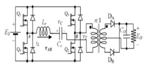
Fig.3 Basic power circuit
