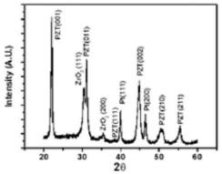
**Fig 2** XRD Graph of PZT sample (un doped) fabricated by conventional methods
