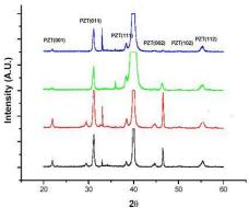
**Fig 4** Comparative XRD Graph of PZT sample (un doped) fabricated by Sol-Gel technology. <u>Blue (</u>PZT Conventional Method), <u>Green</u> (by Sol-Gel Method), <u>Red</u> (PZT with 7% Mg Doping), <u>Black</u> (PZT with composite composition of 7% Mg, and 2.75:1 La/Va)
