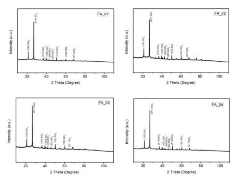
Figure 3: X-ray diffraction pattern (XRD) of Fly ash
