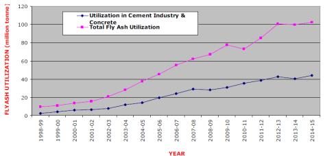
**Figure 2: progressive utilization of fly ash by Cement Industry for the period from 1998-99 to 2014-15** (Source: Central Electricity Authority, annual report, 2014-15)
