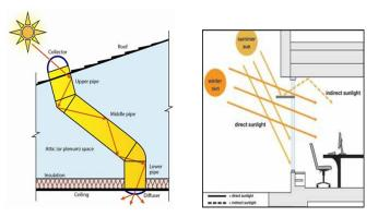
The availability of light within a building depends on its platform, orientation, the location and size of opening. Because of variation in outdoor lighting levels, it is difficult to calculate interior lighting. The ratio of indoor illumination (Ei) to the corresponding outdoor illumination (Eo) in percentage is called as Daylight Factor (D.F.).
