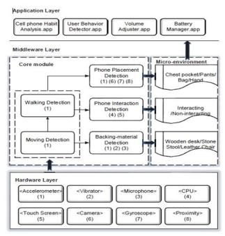
Fig -1: System architecture
