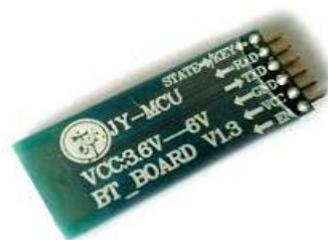
A Bluetooth module is widely used with Microcontroller to enable Bluetooth communication. This module can be interfaced using the UART in 8051 microcontroller where the data are transmitted in the form of packets. The pins TX and RX pin of the HC-05 form the path for data transmission and reception. These TX pin of HC-05 must be connected to the RX pin of 8051 and vice versa. Whereas the key pin of the module is used to set the password for pairing the module with our devices.
