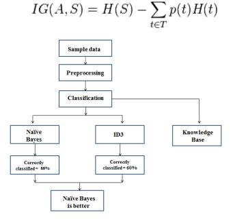
The above flow chat depicts that we have collected the sample dataset from the institute and preprocessing on the data is done. Classification techniques like Naïve Bayes and ID3 algorithm are used to predict the output of the candidates being placed in upcoming placement procedure.
