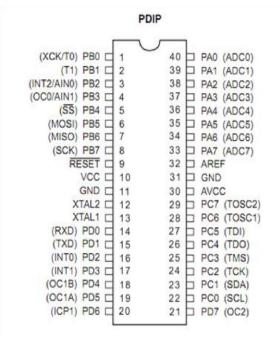
ATmega16 is an 8-bit high performance microcontroller of Atmel's family with low power consumption. Atmega16 is based on enhanced RISC (Reduced Instruction Set Computing) architecture with 131 powerful instructions. Most of the instructions execute in one machine cycle. Atmega16 can work on a maximum frequency of 16MHz.
