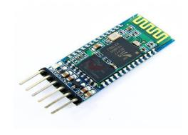
We are using a HC05 Bluetooth module at the receiver circuit so as to receive the command from the application and deliver it to the microcontroller where various command is already fed to it.
