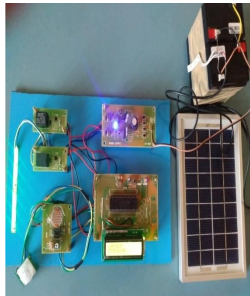
Fig 5:On Board Unit diagram
