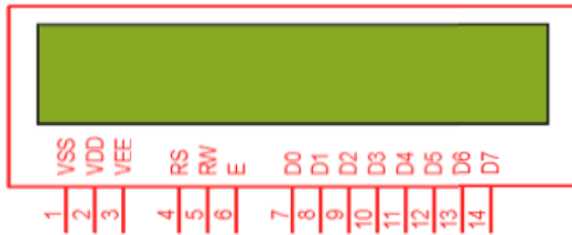
Fig 3: Schematic Diagram for LCD
