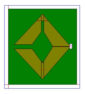
Fig. 1.Simulated Geometry of Proposed Antenna
