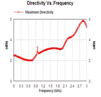
Fig.8. Directivety vs frequency graph
