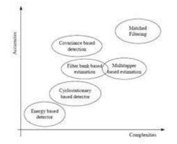
Fig 2:Spectral sensing methods for cognitive radio
