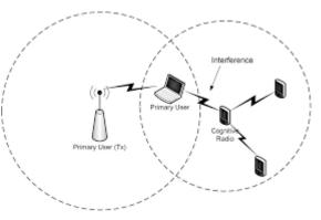
Fig 3:Spectrum sensing in cognitive radio
