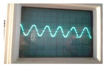
Fig 5. 12v AC (output of 230v/12v transformer)
