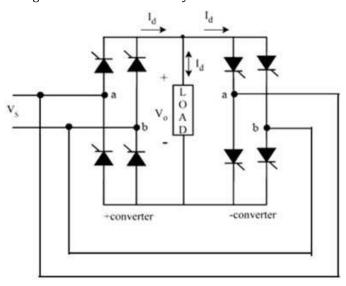
Fig2: 1 phase to 1 phase cycloconverter
