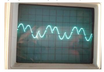
Fig 7 output at load for frequency F=16.66 HZ ie F/3
