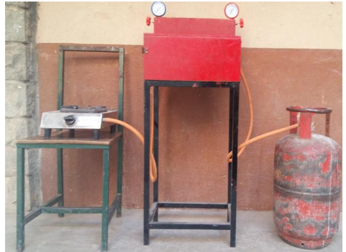
Fig.-2: Actual Setup of LPG Refrigerator
