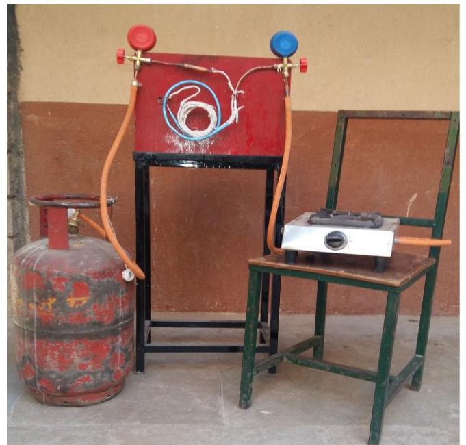
Fig.-3: Actual Setup of LPG Refrigerator
