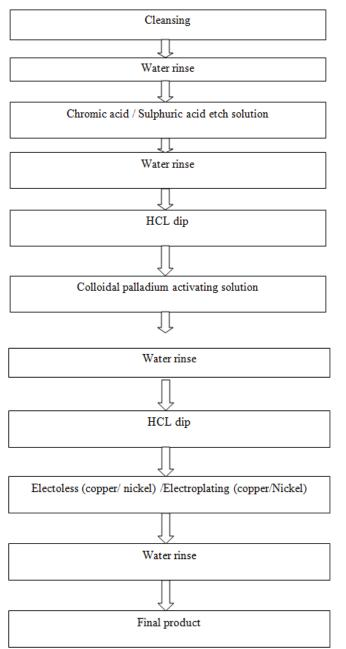
Fig -1: Procedure followed while doing electroplating
