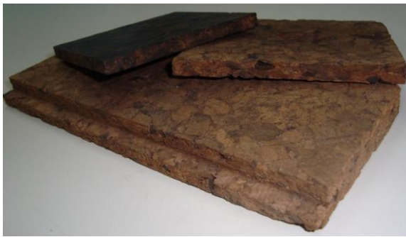
Fig 3 Samples of different densified insulation corkboard (ICB) materials [4]
