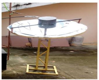
Fig -1: Parabolic dish collector
