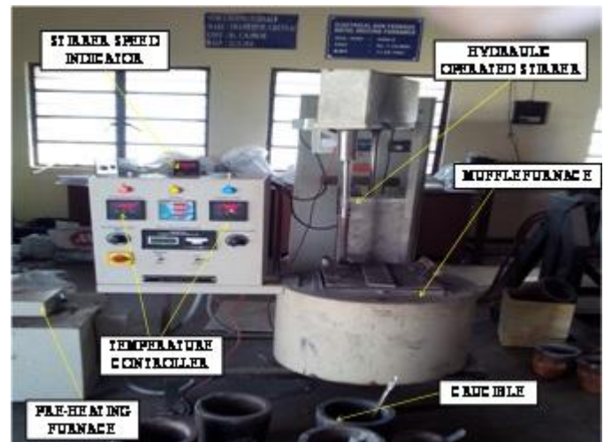
Fig - 6: Stir Casting Setup Arrangements
