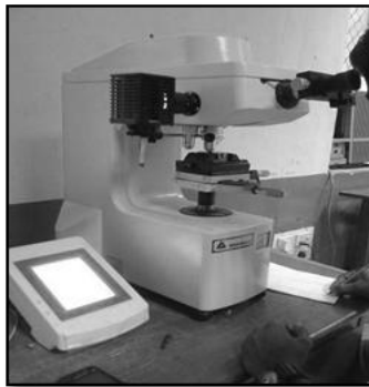
Fig -8: Testing the weld specimens in Vickers Hardness tester
