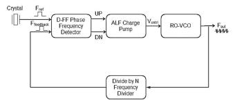
Fig -2: Block Diagram of Modified PLL
