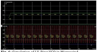
Fig -6: Simulation of LV-Ring VCO in Microwind
