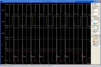
Fig-9: Simulation of D-FF TSPC Flip-Flop in Microwind
