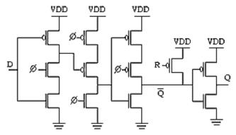
Fig-7: Negative Edge Trigger TSPC Flip-Flop
