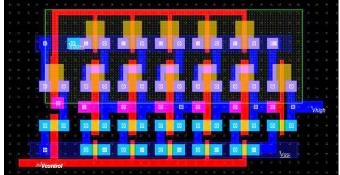
Fig -5: Layout of LV-Ring VCO in Microwind
