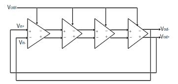
Fig -4: 4-stage Delay Cells in RO
