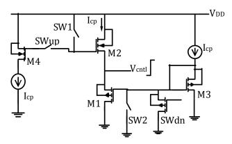
Fig -3: Schematic of MSCC Charge Pump
