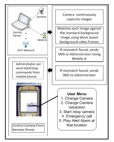
Fig 1. System Architecture
