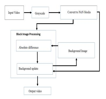
Fig 2. Flowchart to detect motion of an object
