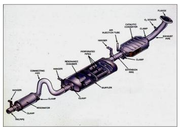
Fig 1 : Exhaust system in automobile
