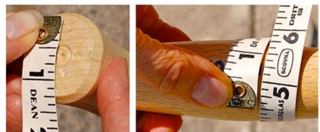
Fig -2. Handle diameter and circumference of the trowel
