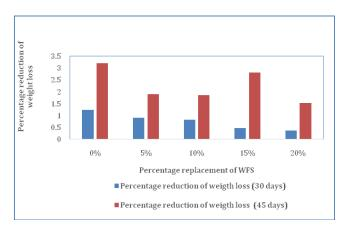
**Fig-5**: Weight loss due to sulphate attack when immersed in 5% solution of sodium sulphate.
