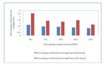
**Fig-6**: weight loss due to sulphate attack when immersed in 10% solution of sodium sulphate.
