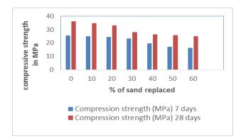
**Fig-1**: Compressive strength of concrete with varying percentage of waste foundry sand.
