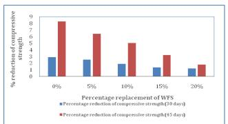
**Fig-4:** variation of compressive strength after sulphate attack immersed in 10% solution of sodium sulphate.
