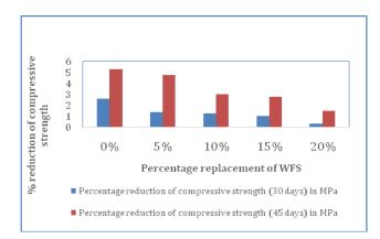
**Fig-3**: variation of compressive strength after sulphate attack immersed in 5% solution of sodium sulphate
