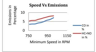
**Chart No-2:** Graphical representation of Speed Vs Emissions with Catalytic converter without Air-box.
