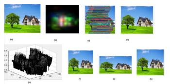
Fig 3. working steps of proposed method. (a) Original Image (b) Saliency map (c) Pixel grouping based on seam searching (d) Coherence filter (e) Assignment of scaling factor. After pixel fusion
