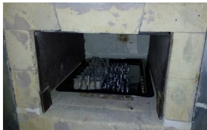
Figure 2: Specimens inside the furnace
