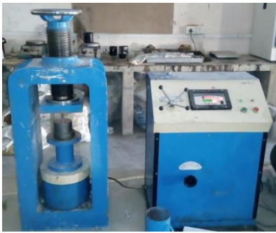
Figure 2. Uniaxial compression testing machine with die under compaction
