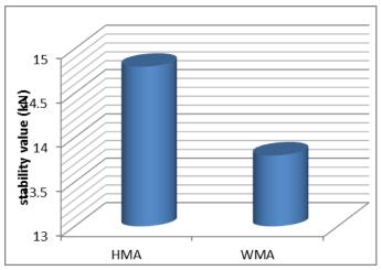
Figure 4.1: Stability value comparison between HMA and WMA
