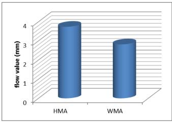
Figure 4.2: Flow value comparison between HMA and WMA
