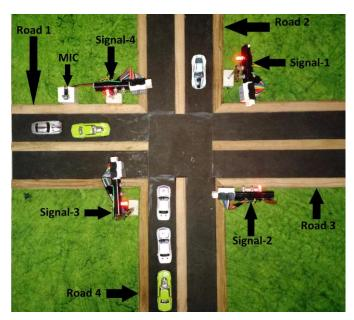
Fig. – 2: Model platform with cars used for simulation
